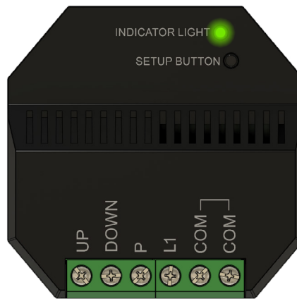
Green flashing Indicator Light Touchlink Commissioning Mode
